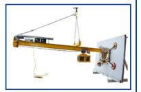
angle of inclination adjustable via movable counterweight with built-on moving gear for rechargeable battery operation
